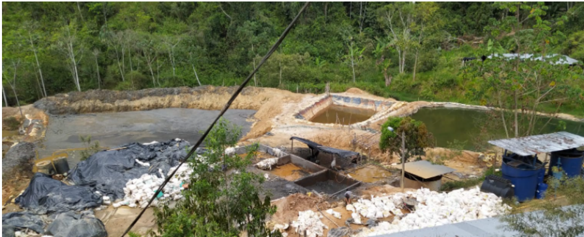
Figure 12. Panoramic view of pools or tailings, where the inert tailings material is located. Source: Pure Earth, 2023.
