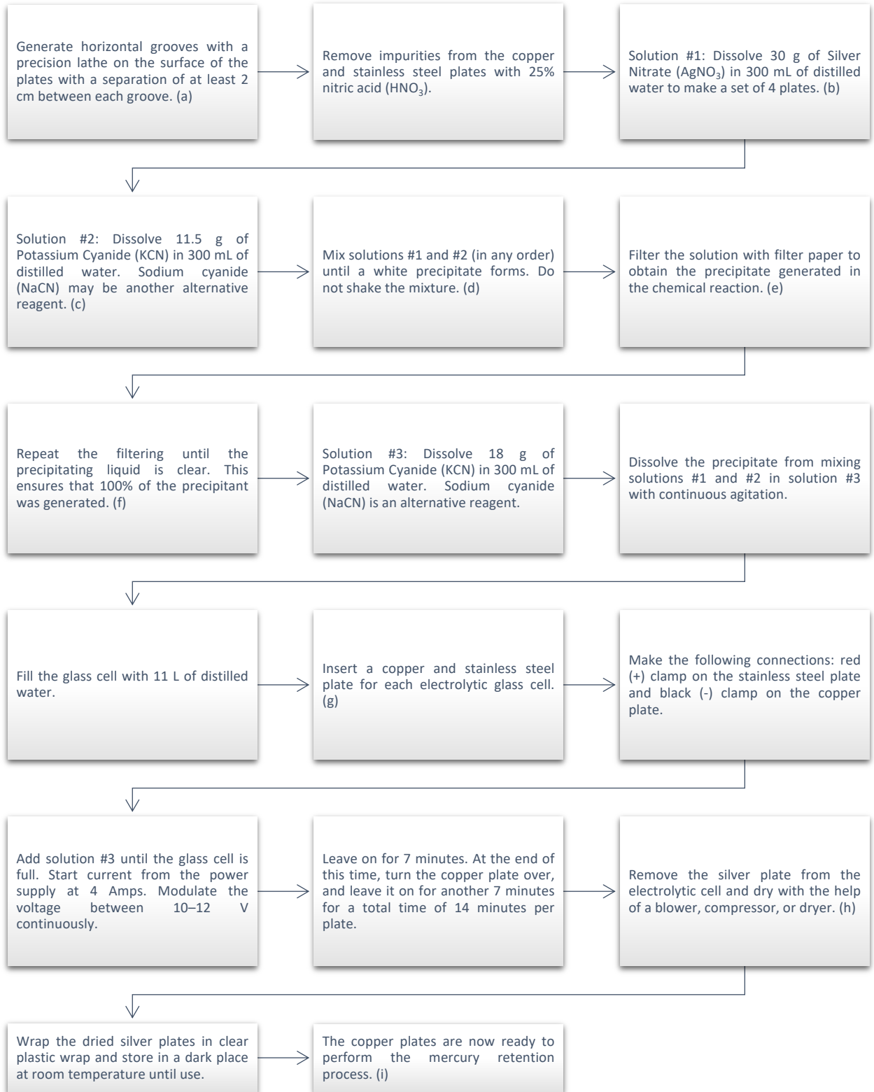
Figure 1. Procedure for the preparation of a set of 4 copper plates. Source: Pure Earth, 2023.
