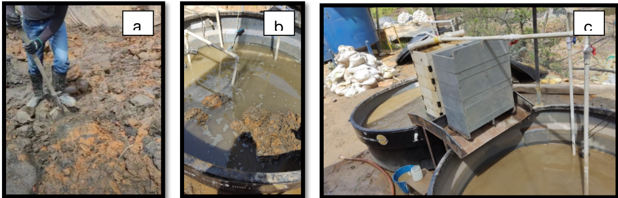
Figure 9. Stages of the pilot tests; a) material loading, b) preparation of tailings slurry solution, c) ignition of pumping equipment. Source: Pure Earth, 2023.
