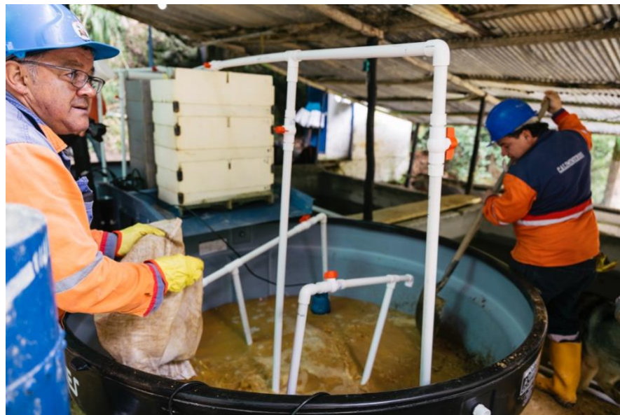
Fig. 2: Miners in Santander learn to use the copper plates technology to clean mining tailings of mercury.
